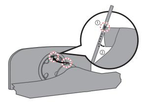
**3** Secure the base to the stand column with the four short screws (provided).
